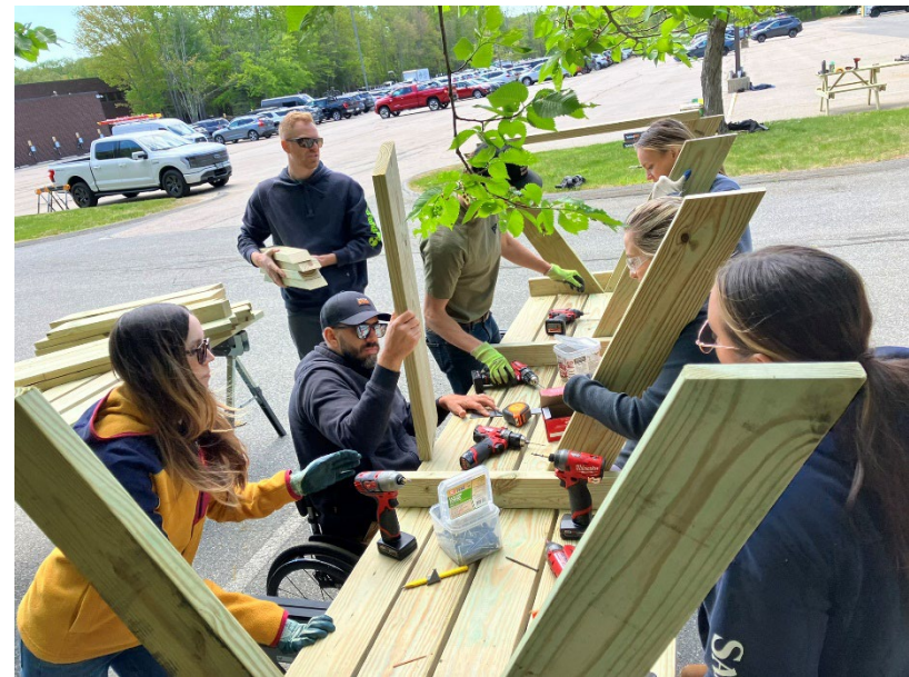
Picture 2: Legs being secured to table stays.
