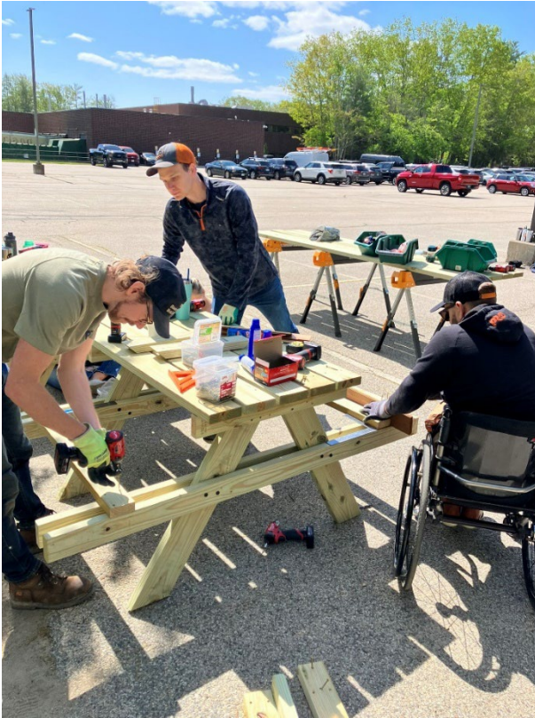
Picture 7: Bench Supports being centered, spaced, and secured.
