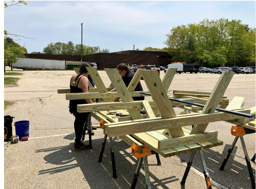
Picture 6: Angled Braces in center of each sitting compartment
