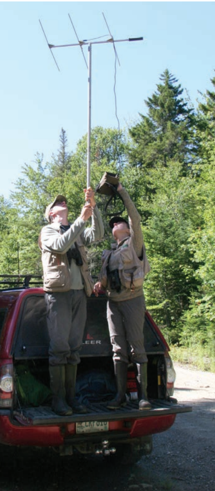
8. Hand-held receivers and directional antennas help to locate the transmitting fledglings. Photo by Dyanna Smith.
